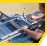
The Ladder Rack Clamp ensures safe and easy transportation of most ladders on a motor vehicle, freeing up interior vehicle space.
